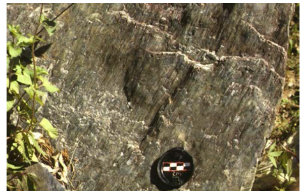
Slickenfibres on a fault plane. The fault surface would be measured as a plane; the slickenfibres as a line. Other surfaces, such as the movement plane , can be calculated from these two measurements.
