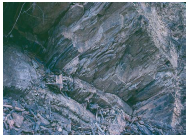
Linear 'pencils' formed by bedding/cleavage intersection in deformed mudstone. The bedding and the cleavage would both be measured as planes. The intersection line between them (which forms the 'pencils') could be calculated from these two measurements, but would be better measured directly in the outcrop as a line.
